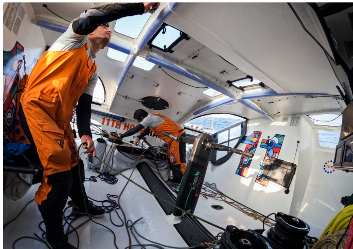
The fully enclosed cockpit of the Malama protects the crew as the boat sails at speeds up to the thirty knots in ocean conditions that can include 40 foot waves, 60 knot winds, and temperatures in the mid thirties.
