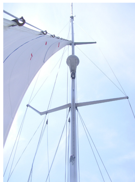
The rouge wave that hit Tenacity caused significant damage to the rig; the boom broke in half and the starboard spreader was bent into a V shape.
