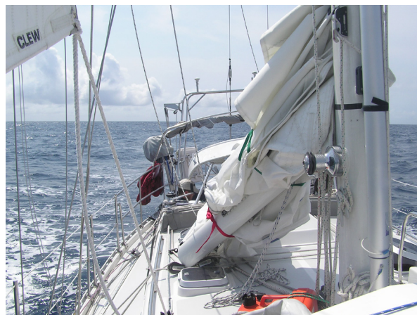
The rouge wave that hit Tenacity caused significant damage to the rig; the boom broke in half and the starboard spreader was bent into a V shape.
